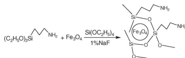
Fig. 1. The formation scheme of MS-1 carrier.
